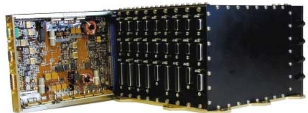
Power Control and Distribution Unit (PCDU)
