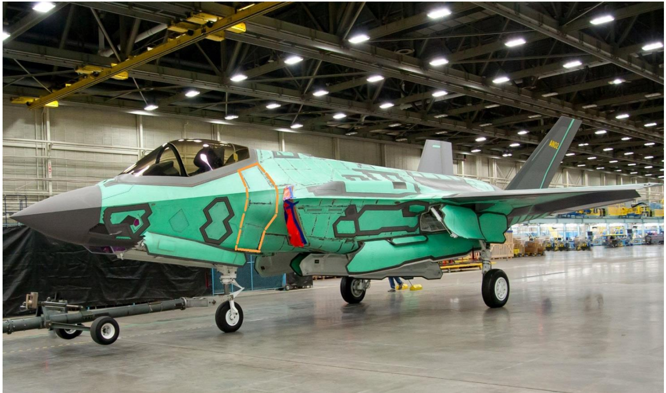
Figure 9 Location of belly band on the F-35A
