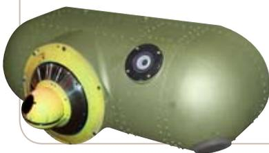
Illustration showing the installation of the CHASE Pod which hosts all of the missile warning sensors and laser-based Directional Infrared Countermeasures, DIRCM.
