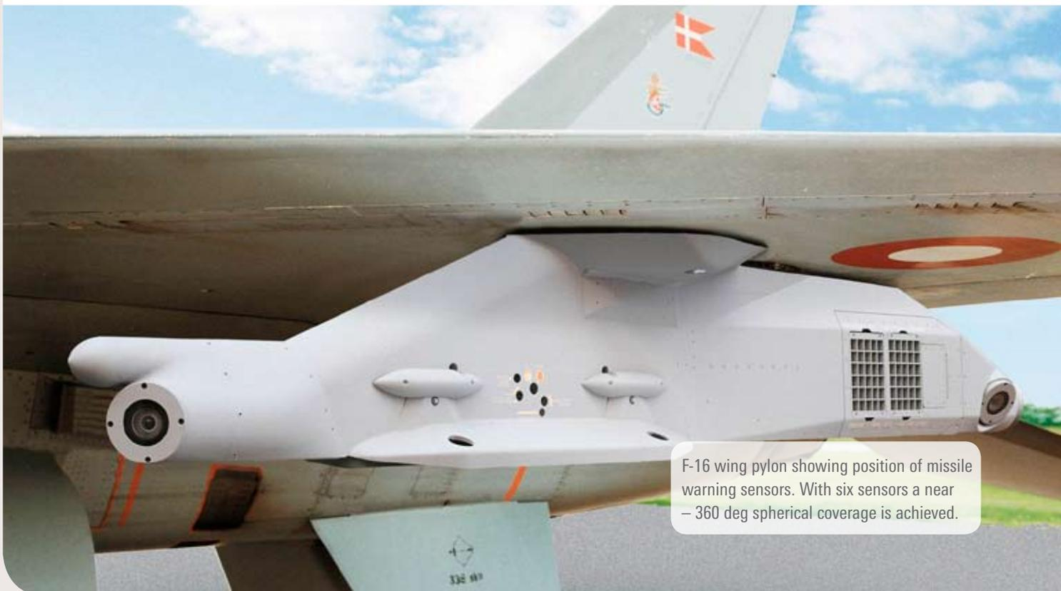
F-16 wing pylon showing position of missile warning sensors. With six sensors a near - 360 deg spherical coverage is achieved.
