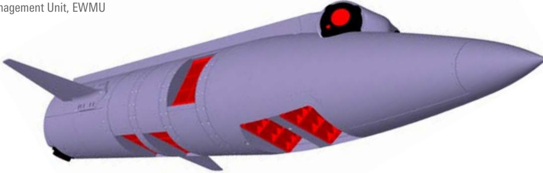
Modular Countermeasures Pod (Sketch) for RAF Tornado GR4 with missile warning sensors and flare magazines. Modules can be rotated in 15 deg increments to obtain optimal firing direction.
