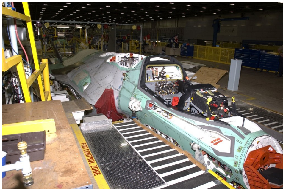
Figure 6 the sliders used to operate close the aircraft. The picture shows sliders in the final assembly area, however, the sliders are identical in the wing manufacturing ( http://www.jsf.mil/images/gallery/sdd/f35_manufacturing/b/sdd_f35manfb_013.jpg )
