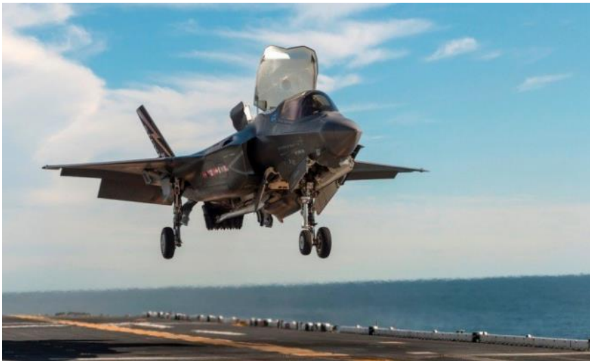
Figure 2-6: F-35B Short Takeoff/Vertical Landing with lift fan and swiveled engine [2]
