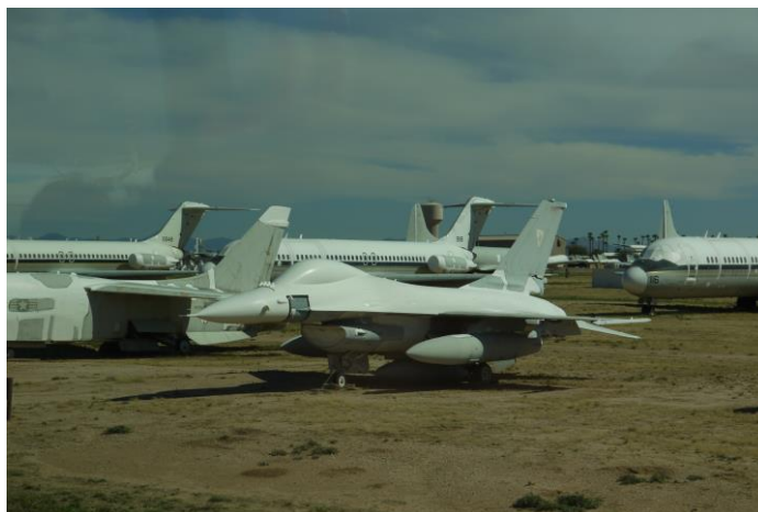
Figure 4-10: The characteristic white coating serving to protect the aircraft from the heat, sun and dust of the Arizona desert, on a decommissioned F-16 Fighting Falcon at the AMARG at Davis Monthan Air Force base. Most of the decommissioned F-16 aircraft will be converted into remote controlled target drones for F-35 live targets.
