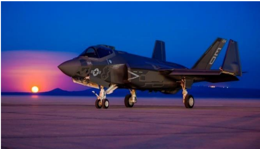
Figure 2-7: F-35C Carrier Variant (CV) with folded wingtip sections and robust landing gear [2]
