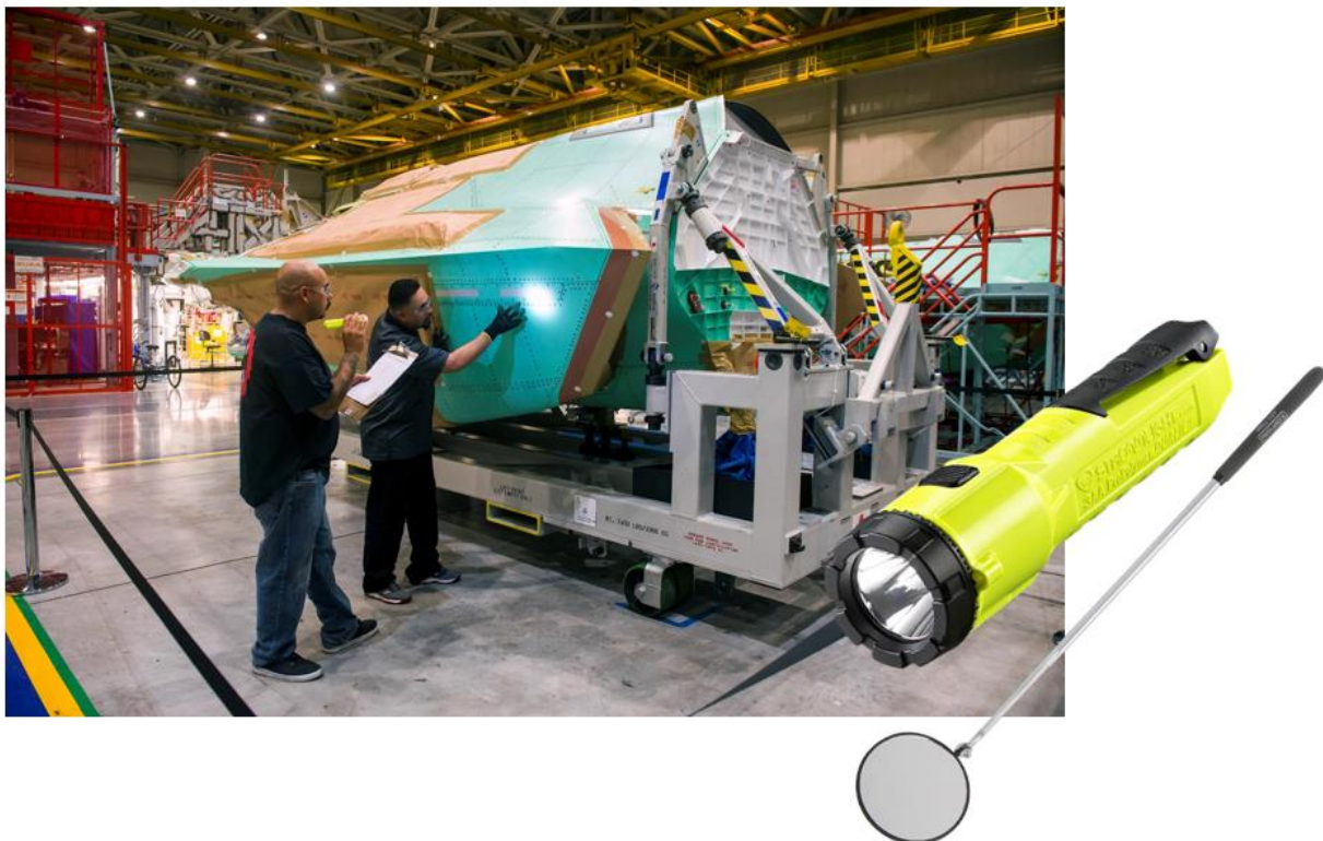
Figure 3-13: Manual inspections of a F-35 centre fuselage at Northrup Grumman similar to those taking place in all aircraft manufacturing operations at Lockheed Martin Aeronautics [5]. Copyright: Northrup Grumman Photo
