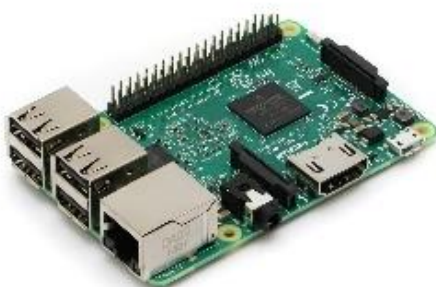
Figure 3-6: Raspberry Pi 3B microcomputer used for video capture and machine vision.
