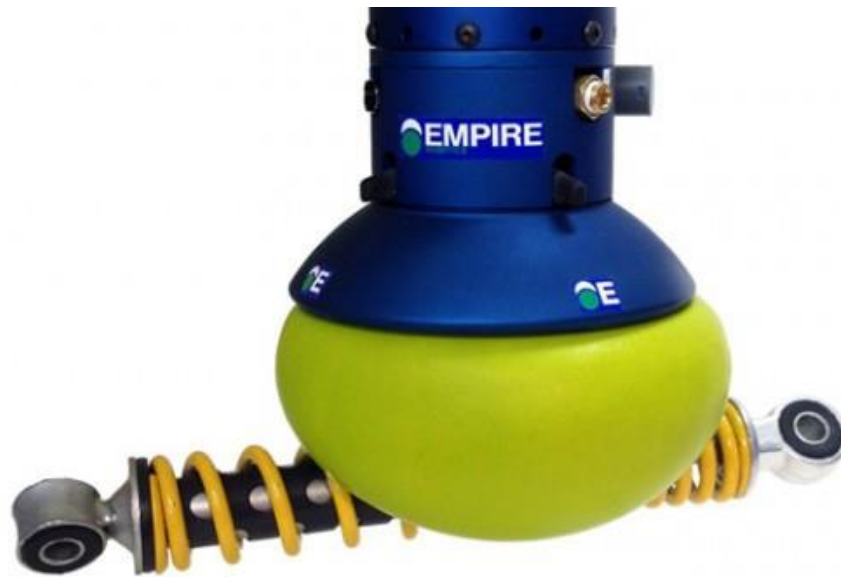
Figure 3-11: A Universal Gripper picking up a spring and a shock absorber assembly [3].
