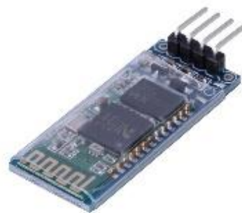
Figure 3-8: HC-05 Bluetooth Master-Slave module for radio communications for example with a smart phone or tablet computer.
