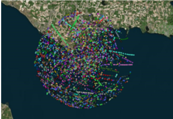
FIGURE 7. Summary of tracked targets before application of classification. In total, 1.48 million track updates were recorded and summarised in this image.
