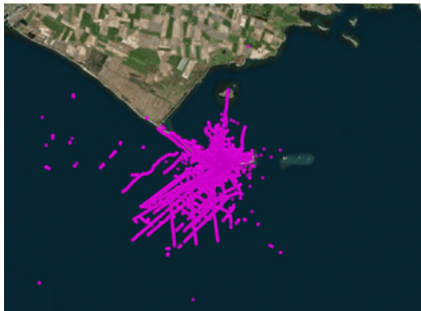
FIGURE 8. The tracked targets the radar automatically classified as drones. The number of track updates is now 19,460 and illustrates the actual drone trajectories.
