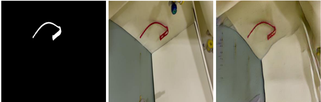
Figure. 1: Image and mask of a mock-up bay to illustrate how the cGAN is used. Left: Labeled mask image. The white area is FOD and the black area is background. Middle: “Real” image of the mock-up F-35 bay. Right: cGAN generated image using the mask to the left.
