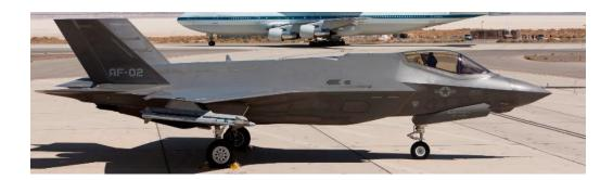
• **F35B (STOVL)** This version is made for the Marine Corps and is the first supersonic aircraft that is able to take off on a short runway and land vertically. This means that it can land and take off on smaller ships. The STOVL can be seen in the picture below
