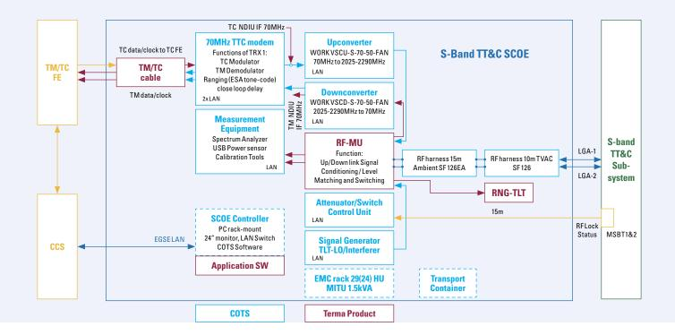
Terma's TT&C SCOE (Telemetry, Tracking & Control-Specific Check-Out Equipment) for testing the satellite platform TT&C subsystem or, at unit level, the transponder (comprising a Telecommand Receiver and Telemetry Transmitter) is based on commercial off-the-shelf (COTS) instruments and a 70 MHz IF TTC modem (IMBU: IF Modem and Baseband Unit), and has been designed for highly-accurate automated measurements.
